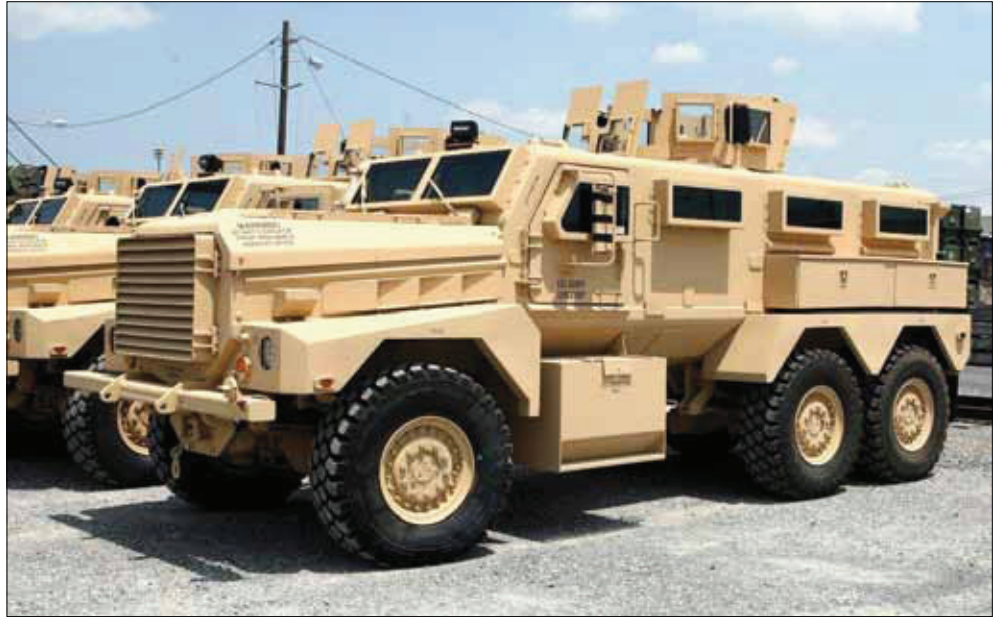
After final paint, this is the final result from the Cougar to JERRV conversion. It is now waiting to be sent to the customer. (Army Photo)
