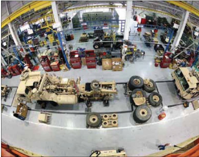
The primary assembly line in the maintenance facility was converted to accommodate reset of PATRIOT Prime Movers. The PATRIOT projects at the depot continue to be a prominent source of work. (Army Photo)
